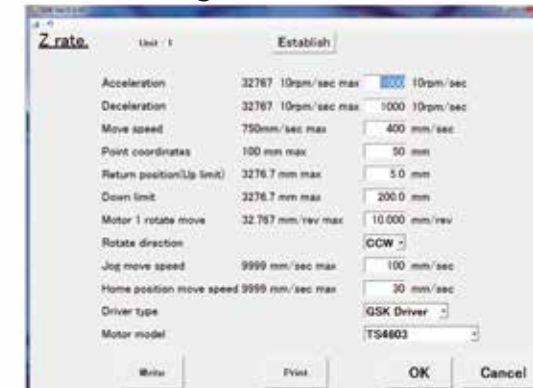
Screen for setting the details of Z-axis motor.
