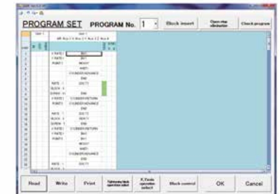
Screen for setting the combination of behaviors related to tightening (socket matching, temporary inversion, final tightening) for each axis tightening, final tightening) for each axis.
