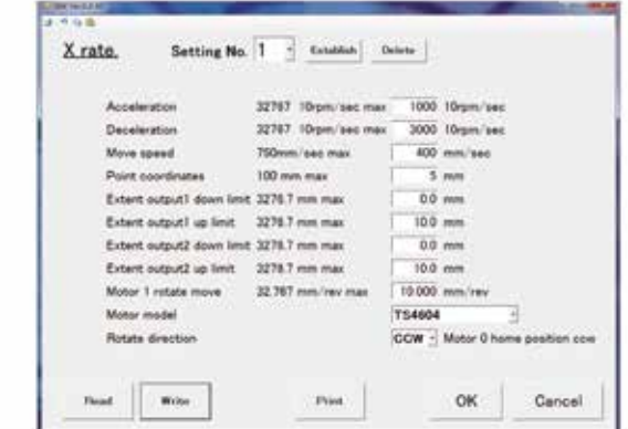
Screen for setting the details of X / Y-axis motor.
