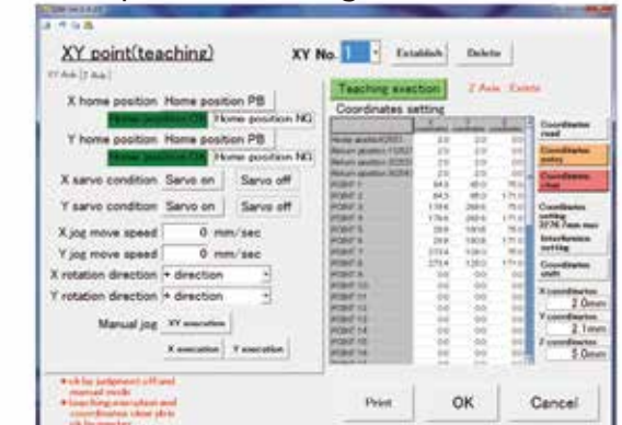
Screen for setting (teaching) the tightening coordinates.
